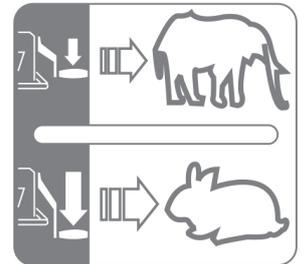
Maximum splitting force at lower speed for splitting particularly hard or stored logs or at the beginning of the splitting process → middle position of the operating handle.
