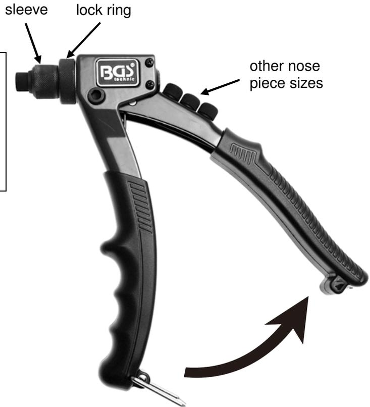
Adjust appropriate working stroke to match with different nose piece size. Rivet can be snapped after 3 - 4 times.
