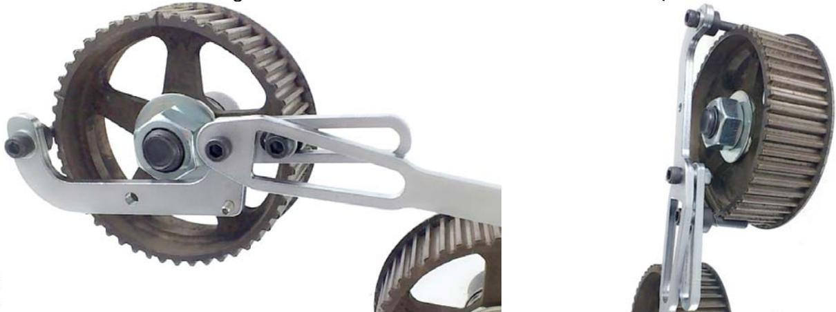
Hold the counter holding wrench when loosening or tightening by hand, or if possible on the second camshaft sprocket as shown in the figure.
