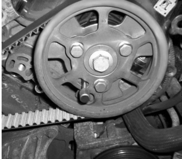
LR/Jaguar 3.0TDV6 and PSA 2.7/3.0D HDi Insert 1 x (D) in the left hand camshaft/sprocket (Fig.8), and the other (D) in the right hand camshaft/sprocket. (Fig.9)
