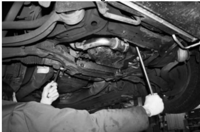
9. NOTE: The 'pin' of (B) (manual transmission) Locking Tool is offset (Fig.A), and once it has been inserted, the Locking Tool is fixed in position by securing it at the starter motor bolt position.
