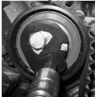
15. Using a suitable Sprocket Holding Tool to counter hold the sprockets, tighten all 6 sprocket bolts to 23 Nm.
