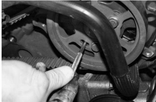
**NOTE:** Reference to left hand or right hand camshaft is as viewed when looking directly at the camshaft sprockets. Check that the belt tensioner is in the correct position - the mark (casting mark) on the tensioner can be seen through the 'cut out notch'.
