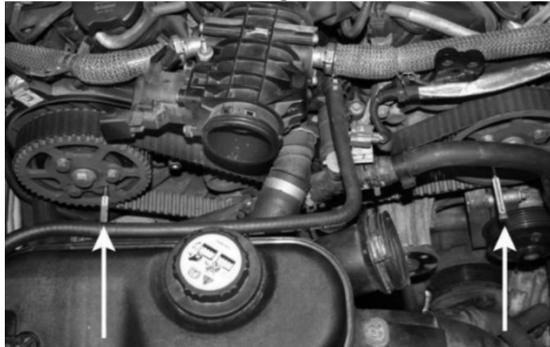
11. Remove the timing belt tensioner and the old timing belt.
