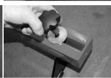
Insert the bolt of the bracket into each side of the engine support.
