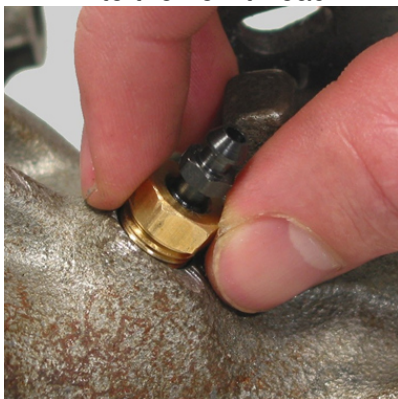
Insert the valve insert into the new thread
