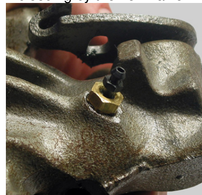
The brake system can now be bleeding by the new valve..
