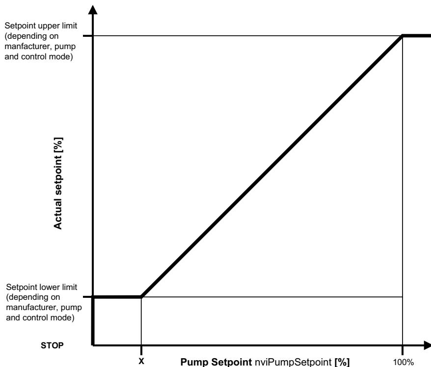
$$X = (\text{Setpoint lower limit} / \text{setpoint upper limit}) * 100\%$$
