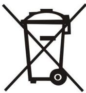
In observance of European Directive 2012/19/EU on waste electrical and electronic equipment and its implementation in accordance with national law, electric tools that have reached the end of their life must be collected separately and returned to an environmentally compatible recycling facility.
