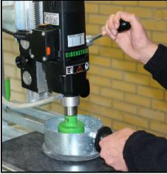
Put the tile or plate you want to drill on the drilling table and adjust it. Fix the workpiece with the hold-down which fulfils the task as a splash guard as well.
