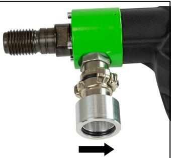
Dust which occurs during your work is hazardous to health. That is why it is advisable to use a deduster (Dust class M) and to wear a dust mask on dry drilling. Place the adapter for the dedusting unit onto the tool's connector and turn into the direction of the arrow up to the stop. As a suitable wet/dry deduster, our DSS 35 M iP is available as add-on. The use of a dedusting system is also a prerequisite for optimal cutting performance of the bit (air cooling).
