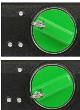
The **ESD 200** is equipped with a mechanical 2-speed oil-bath gearbox. Select the speed according to the drilling diameter (ref. to the tool's identification plate). Loosen the detent bolt on the gear change switch and turn the gear change switch as far as it will go into the faster or slower gear.
