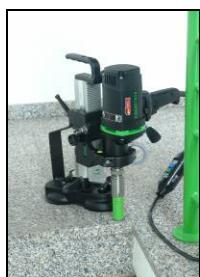
At the beginning, drill very slowly, since the drill bit does only starts cutting with a fraction of the cut surface in the material. If you drill too fast or with too much pressure, the drill bit could get jammed.
