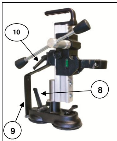
For drilling in niches and corners, the drill column can be swivelled by up to 360°. To do so, open the clamping lever (8), turn the drill column into the desired position and close the clamping lever.
