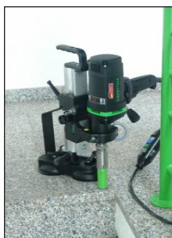
At the beginning, drill very slowly, since the drill bit does only start cutting with a fraction of the cut surface in the material. If you drill too fast or with too much pressure, the drill bit could get jammed.
