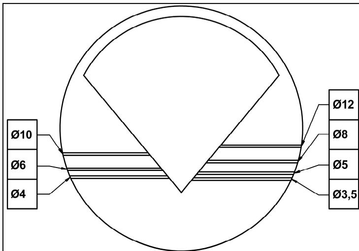
The maximum drilling diameter is 25 mm, whereby there is no centring aid between 12 and 25 mm.
