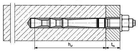
Pre-positioned or push through installation with subsequently pressed filling disk (annular gap filled with mortar)
