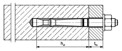
Pre-positioned or push through installation with subsequently pressed filling disk (annular gap filled with mortar)
