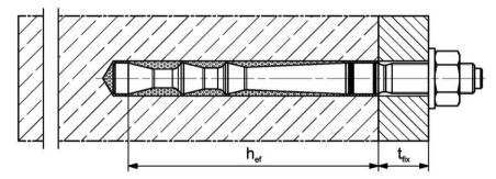
Push through installation not with mortar capsule (annular gap filled with mortar)
