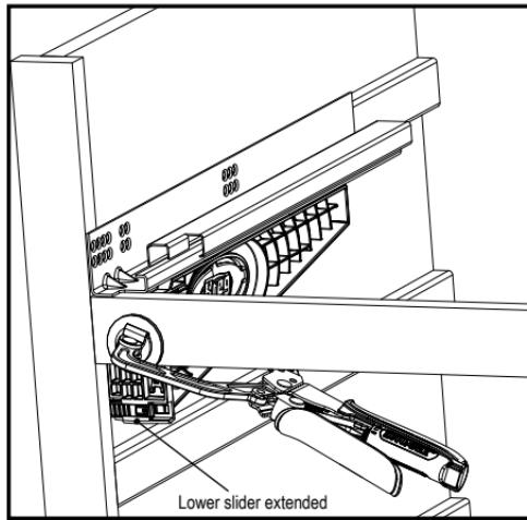
**ATTENTION** Where the inside edges of the face-frame stiles are flush with the inside faces of the cabinet sides, do not extend the Lower Sliders. Clamp the Brackets to the cabinet sides. Make sure the clamp pad bears on the Bracket ribs, not the webbing between the ribs, including the web area with the Kreg logo. Clamping with the clamp pad on the webbing could crack the Bracket.
