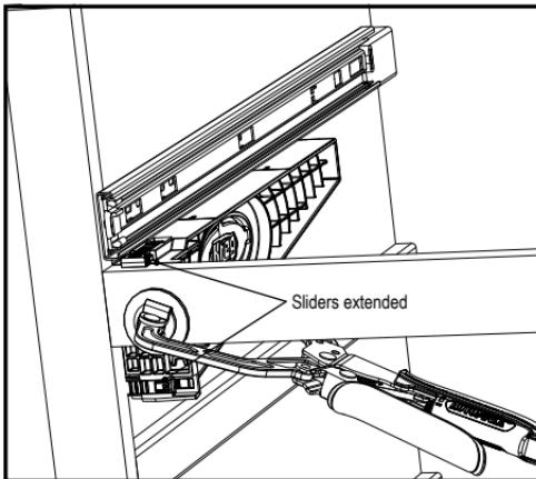
**MOUNTING DRAWER-SLIDE CABINET MEMBERS****Under-Mount Drawer Slides****Position the Brackets**
