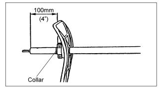
Fit the gear case to the pipe shaft, and securely fix it with one loosening-preventing bolt and two tightening bolts (tightening torque: 5 – 6 N-m).
