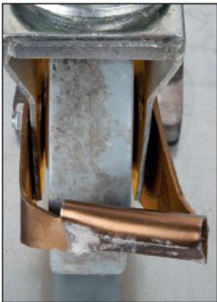
Foot pedal distortion as a result of a significant impact; it is likely the top plate and bearing will be distorted as well.
