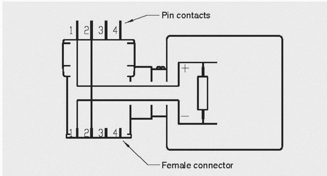
If the transmitter to be connected does not have the negative power terminal on contact 2 and the positive power terminal is not on contact 1, then the assignment of the A-AI-1 angular connector and the external angular connector must be matched accordingly. To do this, open the A-AI-1 angular connector and exchange the wires from contact 1 and contact 2, so that these match the connection of the transmitter to be attached.
