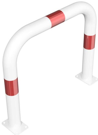
Anti-nudge hoop Ø 76 x 2,6 mm without cross bar to be fixed by plugs, total width: 750 mm, total height: 650 mm, hot-dip galvanized and white coated with red reflecting stripes
