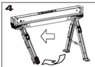
Above the indication "CLOSE 1ST", press the release button and fold down the legs until they are completely unfolded.
