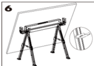
Unfold the support pins to support a plate for cutting.
