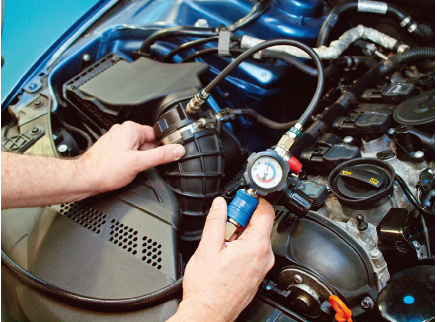
Example shows the tool testing a turbo system intercooler coil for integrity
